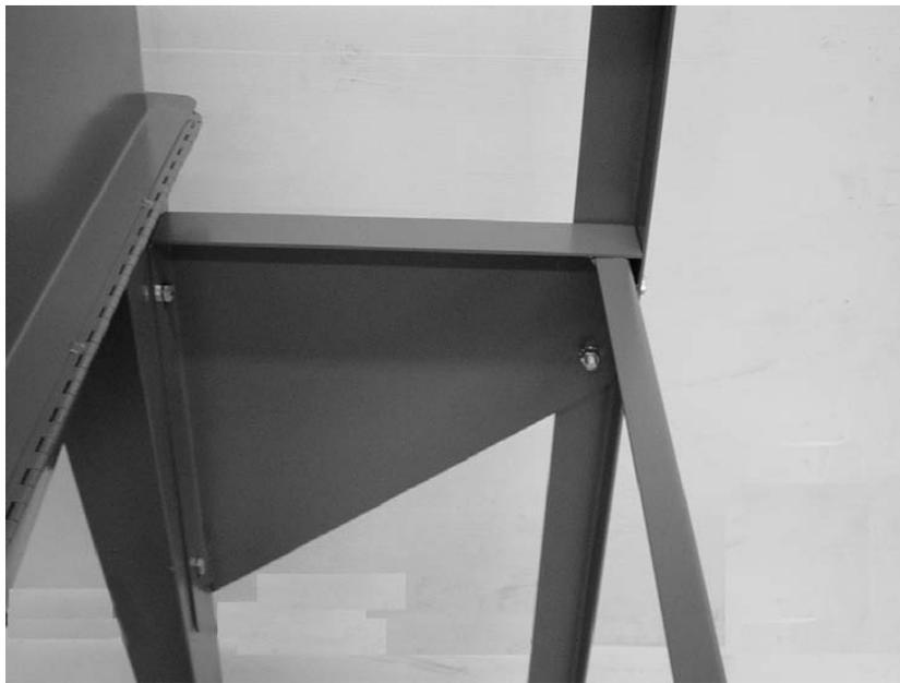
Begin assembly by securing the wide flange of each triangular bracket with (2) 3/8-16 bolts into cabinet legs. Once the triangular brackets are in position on the back of the cabinet, secure the back rack support legs (2) through the narrow end of the triangular bracket with (4) 3/8-16 bolts and nuts into the leg. Attach the horizontal support, with flange on top, to both support legs with (2) 3/8-14 bolts and nuts through legs.
